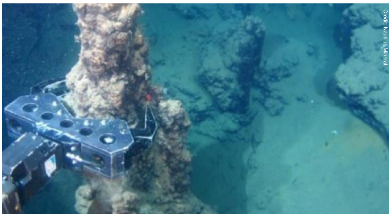
Figure 28: Grab sample of deep-sea thermal vent chimney during exploration
